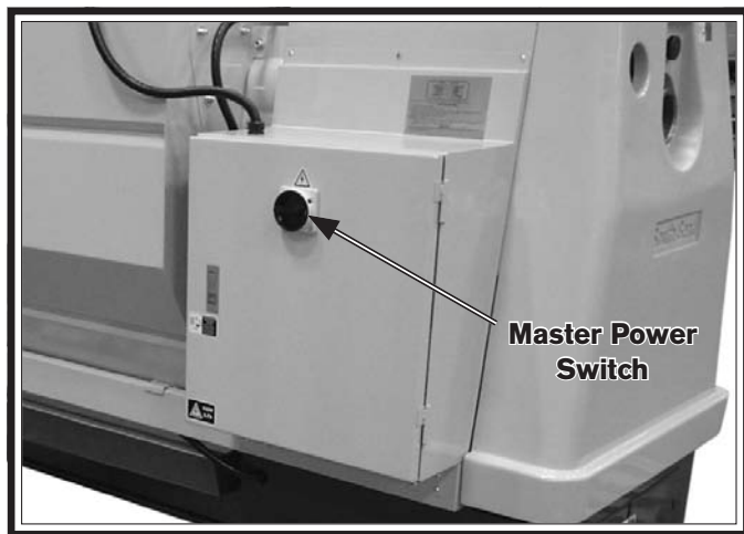
Figure 2. Location of the master power switch.
